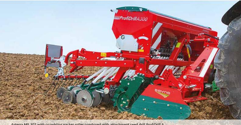
Arterra MS 302 with crumbling packer roller combined with attachment seed drill ProfiDrill A
