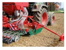
The Terramat and Arterra rotary harrows can also be fitted with track indicators for use with the seed drill. These are operated by a double-acting hydraulic system and fold vertically.
