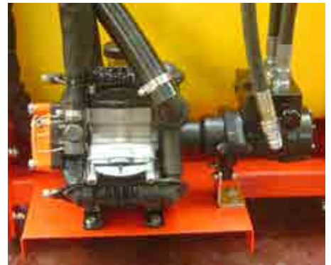
Pomp 120 l/min + hydromotor
