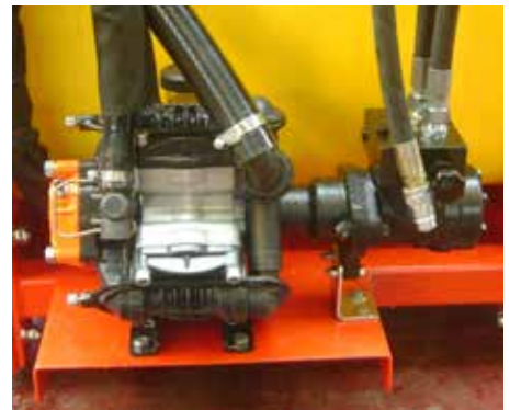
Pumpe 120 l/min + Hydraulikmotor
